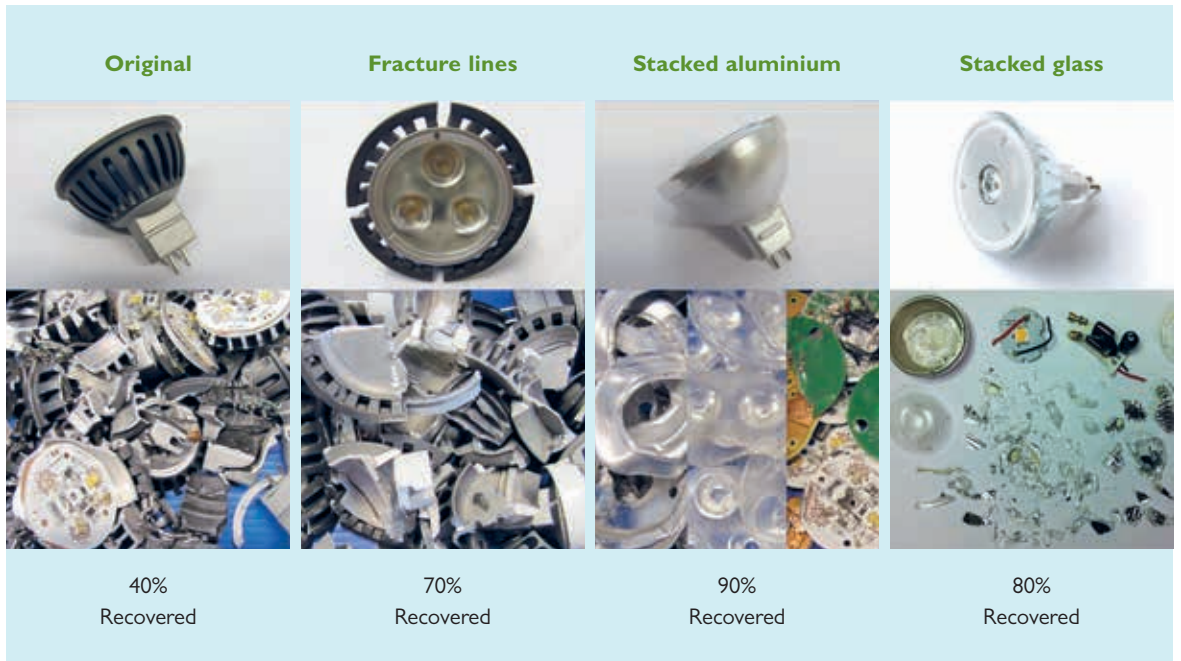
Figure 5. A LED spot light (top left) and three redesigns employing different materials and connections to improve the recycling result. The images at the bottom show typical fragments resulting from a shredding test. Recovered fractions are given in weight-%.
